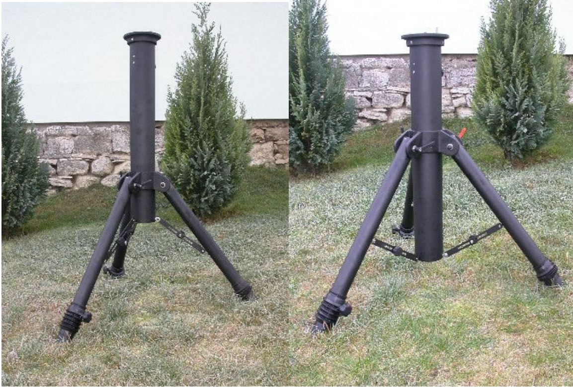
The above photos illustrate the high (left) and low position of the GHS 140 tripod.
